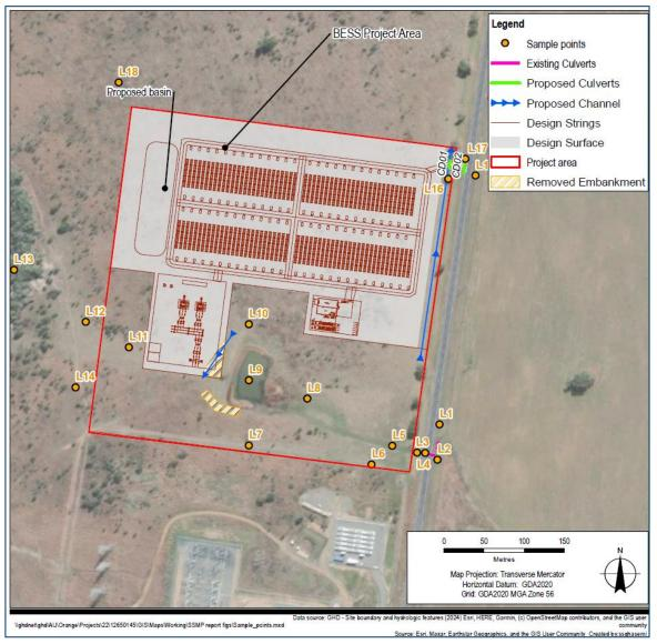
Figure 10 Hydraulic model results sample locations
