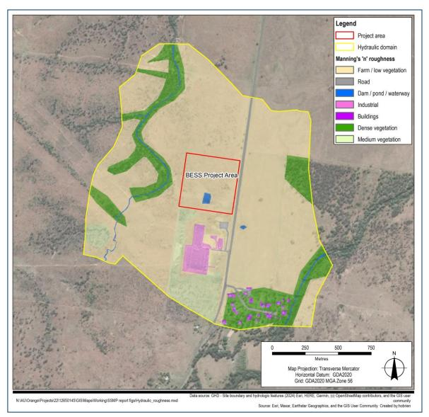
Figure 7 Hydraulic roughness – pre-developed condition
