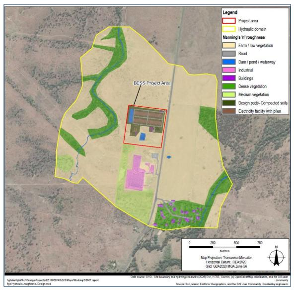
Figure 8 Hydraulic roughness – post-developed condition
