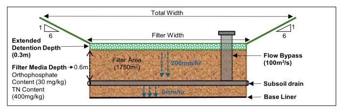
Figure 12 Bio-retention basin typical layout
