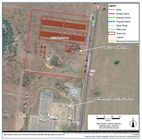
Figure 4 Proposed design drains and culvert
